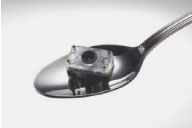
Figure 3 – HHP's IT4000 is a critical Adaptus building block. Implementing a CMOS camera, it is the eyes of the Adaptus technology.
